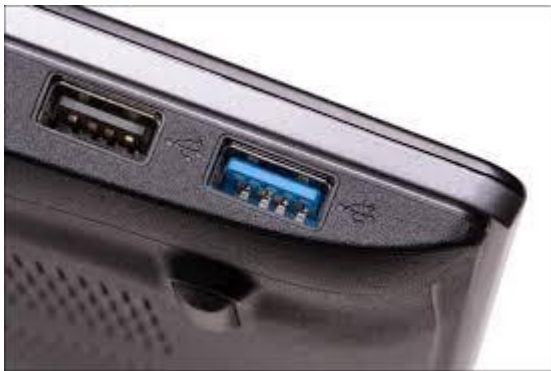
Figure 9: USB2 port (left), USB3 port (blue, right)
